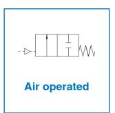
The construction of an air-piloted valve is similar to the direct-operated valve. Instead of using a solenoid and armature to move the position of the internal valve sealing element, it is moved directly by the air pressure supplied to the air pilot port. When the pilot supply is removed, the valve returns to its original position by a return spring.
