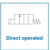
The construction of a direct-operated valve is relatively simple. The internal valve sealing element is directly connected to a plunger or armature. The armature moves when a voltage is applied to a solenoid coil. To generate enough force to create this movement consumes power. When the solenoid is not operated, the armature and sealing element is returned to it's original position by the force provided by a return spring.
