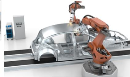
**Schweißen von Automobilteilen**
